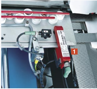
1 The DOUBLE-SHEET DETECTOR is included in all models.
