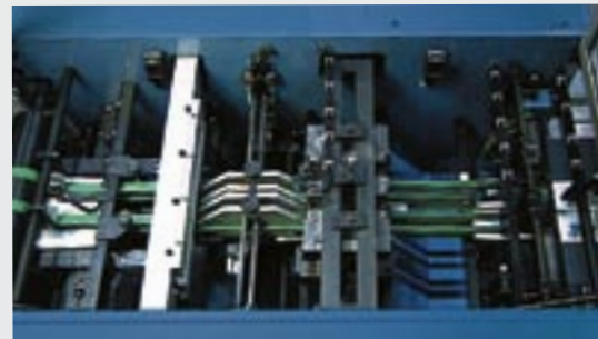
Face trimming; then head, gutter, and foot trimming in three-up production.
